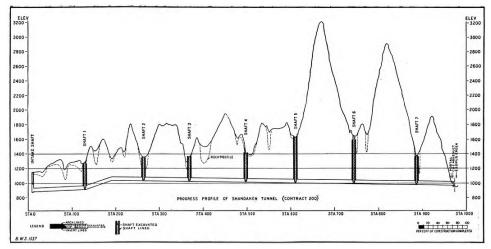
Profile of the Shandaken Tunnel showing the 8 shafts (the intake on the left; the sump and graded tunnel; and the effluent portal). 14th Annual Report of the Board of Water Supply (1/1/1920)
